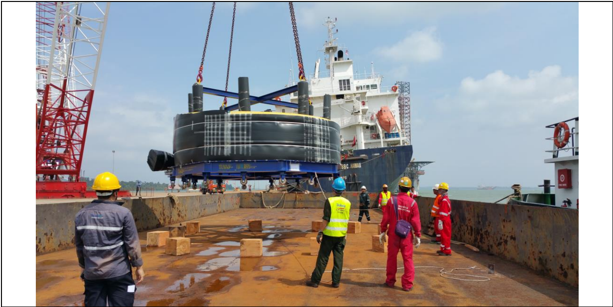
Pic 2: Cargo base is installed with rollers. Customized huge wooden blocks are used to prevent rolling movement and damaged of rollers.
