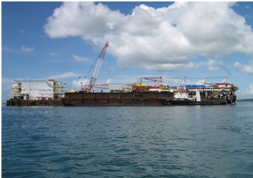
Tug and Barge serves as support, extension and storage for various Oil Rig tools and equipments
