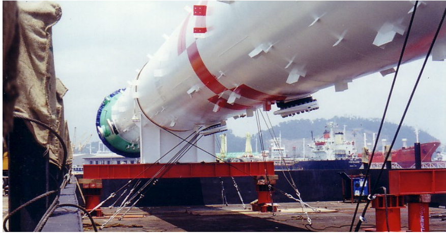
Transportation of Overlength Vessel about 70m length 685 tons
