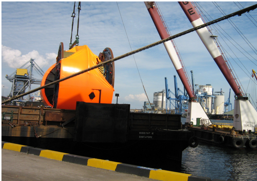
Lifting of Reels Cargo done by utilising Semco floating crane
